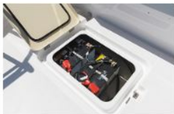
Battery space (stores 2)
