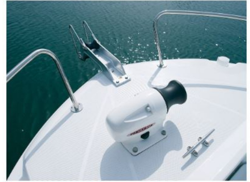
Bow rail (option), navigation light (option), anchor dabit (option), anchor winch (option)
