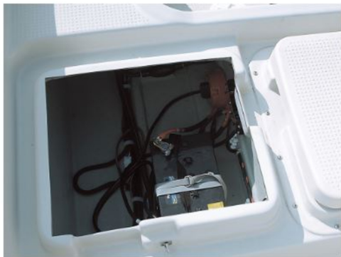
Stern battery space
