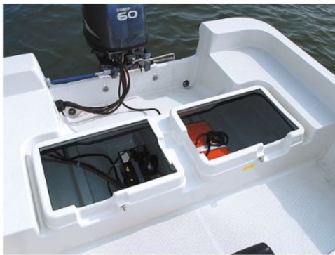
Stern container / fuel tank space
