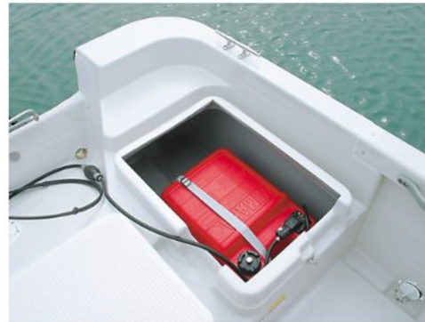
Stern fuel tank space
